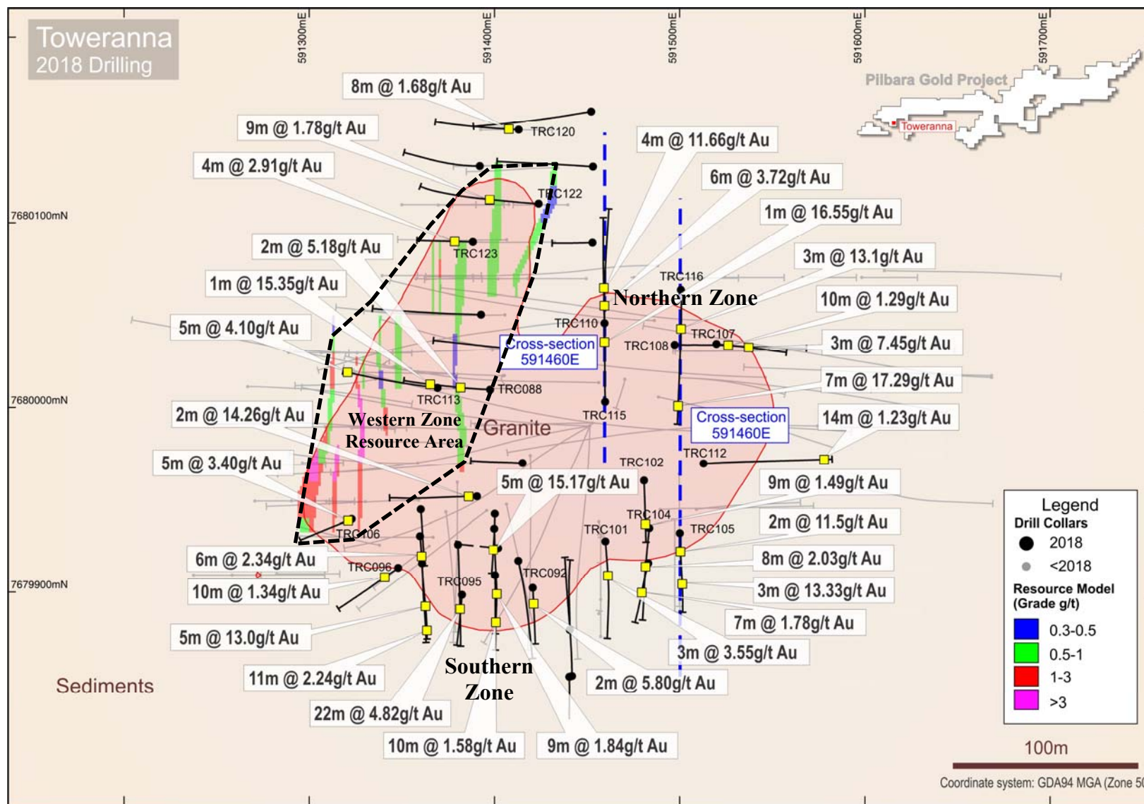
Figure 2 Toweranna – Drilling Plan showing new drill intersections >10gm*m
